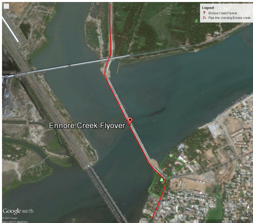
Figure 6.4 – Proposed Pipe Carrying Bridge of Conveying Main across Ennore Creek Parallel to Ennore Creek flyover
